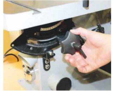
Rack and pinion gearing make tilting the table easy
